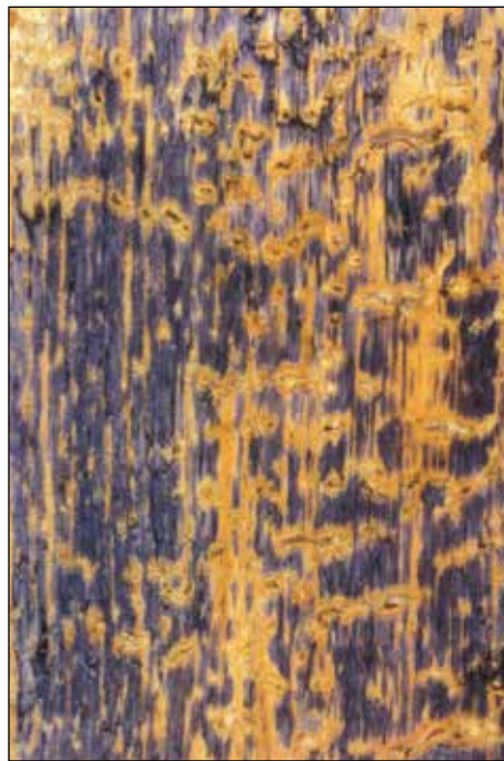
Figure 6. Ganoderma applanatum , the artists conk (top), produces a mottled white rot (bottom left). This decay is a mixture of simultaneous white rot and selective lignin degradation. Black spots in the decayed wood are manganese deposits which accumulate during delignification. The composition of the mottled decay can be differentiated using histological reagents that are applied directly to the surface of the decayed wood. Iodine-Potassium-Iodide / H_2SO_4 stains wood (middle photo at bottom) showing cellulose blue and lignified areas yellow. Another reagent used to identify lignin is phloroglucinol HCl. This stains lignin red while cellulose remains white (bottom right photo).
