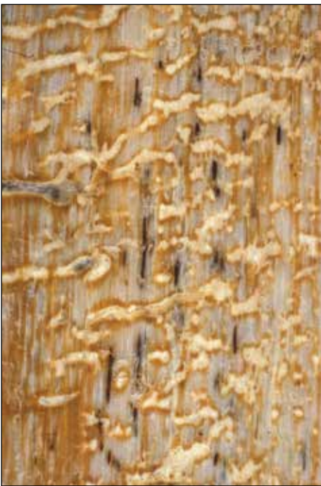
Figure 6. Ganoderma applanatum , the artists conk (top), produces a mottled white rot (bottom left). This decay is a mixture of simultaneous white rot and selective lignin degradation. Black spots in the decayed wood are manganese deposits which accumulate during delignification. The composition of the mottled decay can be differentiated using histological reagents that are applied directly to the surface of the decayed wood. Iodine-Potassium-Iodide / H_2SO_4 stains wood (middle photo at bottom) showing cellulose blue and lignified areas yellow. Another reagent used to identify lignin is phloroglucinol HCl. This stains lignin red while cellulose remains white (bottom right photo).
