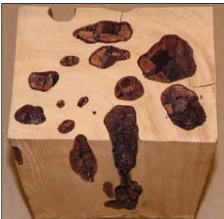
Figure 3. Brown rot fungi usually cause a diffuse attack that is widely distributed in wood. However, some brown rot fungi that attack living cypress, cedar, and other trees with resistant heartwood produce brown rot that occurs in distinct pockets of various sizes. Pecky cypress and pecky cedar are examples.
