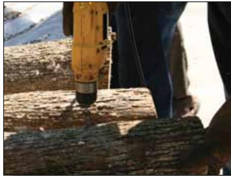
Drilling logs with ordinary drill, note stop collar.
